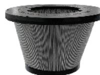
Filtration is provided by a robust polyester cartridge filter. The cartridge is made to maintain a large filter surface area in a compact space. This allows air to pass through even when the filter is dirty. The filter is class M certified (BIA | EN 60335-2-69) and stops particles down to 1 micron, preserving motors and the operator.
