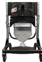
The material is collected inside a sturdy plastic bag called Longopac® that is 20 m long. The sack is rolled below the chamber and is adaptable to any need. The operator, once the sack is filled, can close it above the vacuumed material that has automatically fallen inside, seal it, cut the sack segment with the debris, and dispose of it safely, with no contact between operator and material.
