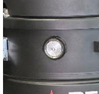
Safety overpressure valve installed on the vacuum chamber
