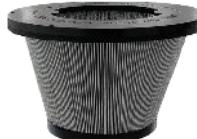
Filtration is provided by a robust polyester cartridge filter. The cartridge is made to maintain a large filter surface area in a compact space. This allows air to pass through even when the filter is dirty. The filter is certified class H (BIA | EN 60335-2-69) preserving the motors and the operator.
