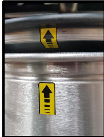
It is possible to lift the container only when the filter unit is correctly positioned.
