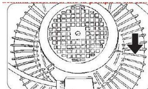
If the rotational direction of the motor is incorrect, use a screwdriver to remove the screw from the power supply plug and invert the two poles, rotating 180°.
